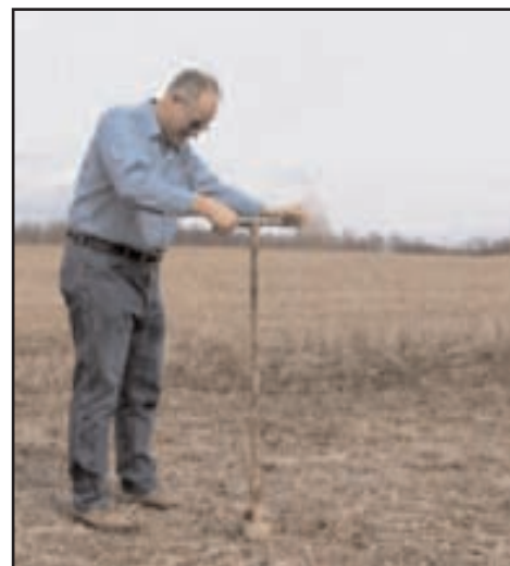
Jim Fridrich, R.S., takes a soil sample at a site for a proposed residential development.
