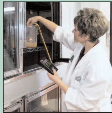
Registered Sanitarian Terri Hillier checks for the correct food temperature in a refrigeration unit at the Inn at Hillen Vale, a residential care facility.
